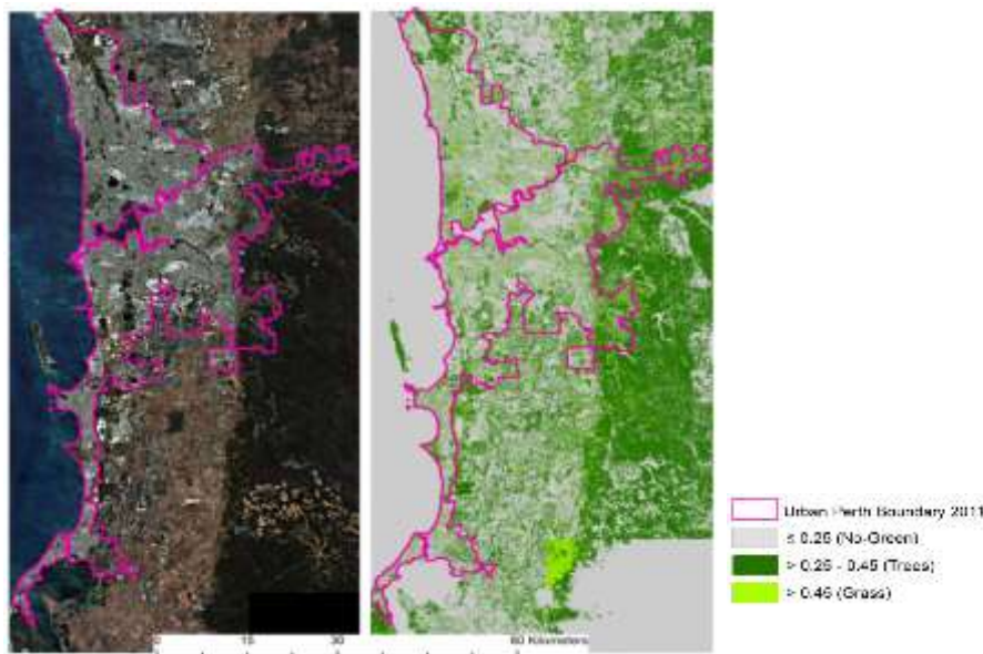
Figure 23: Map of green space for Perth with Sentinel EVI2, 8 December 2016. Map on the left is true colour Sentinel satellite image of Perth; Map on right shows EVI2 values from same Sentinel satellite image.
