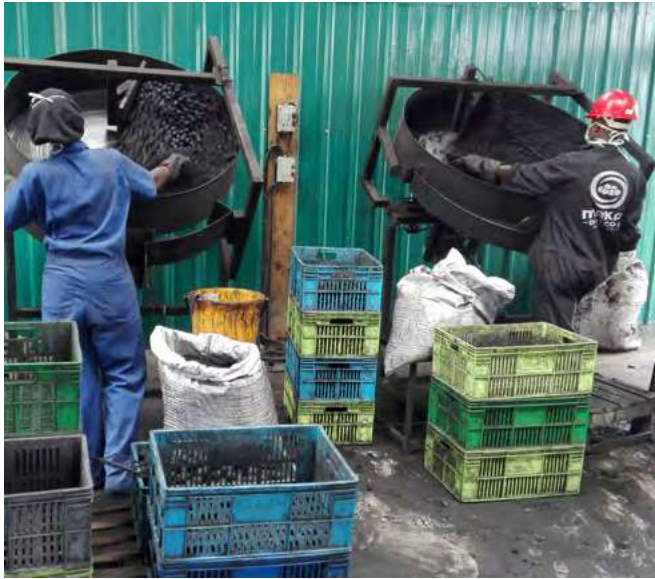
Agglomerator in operation using a rotating drum
