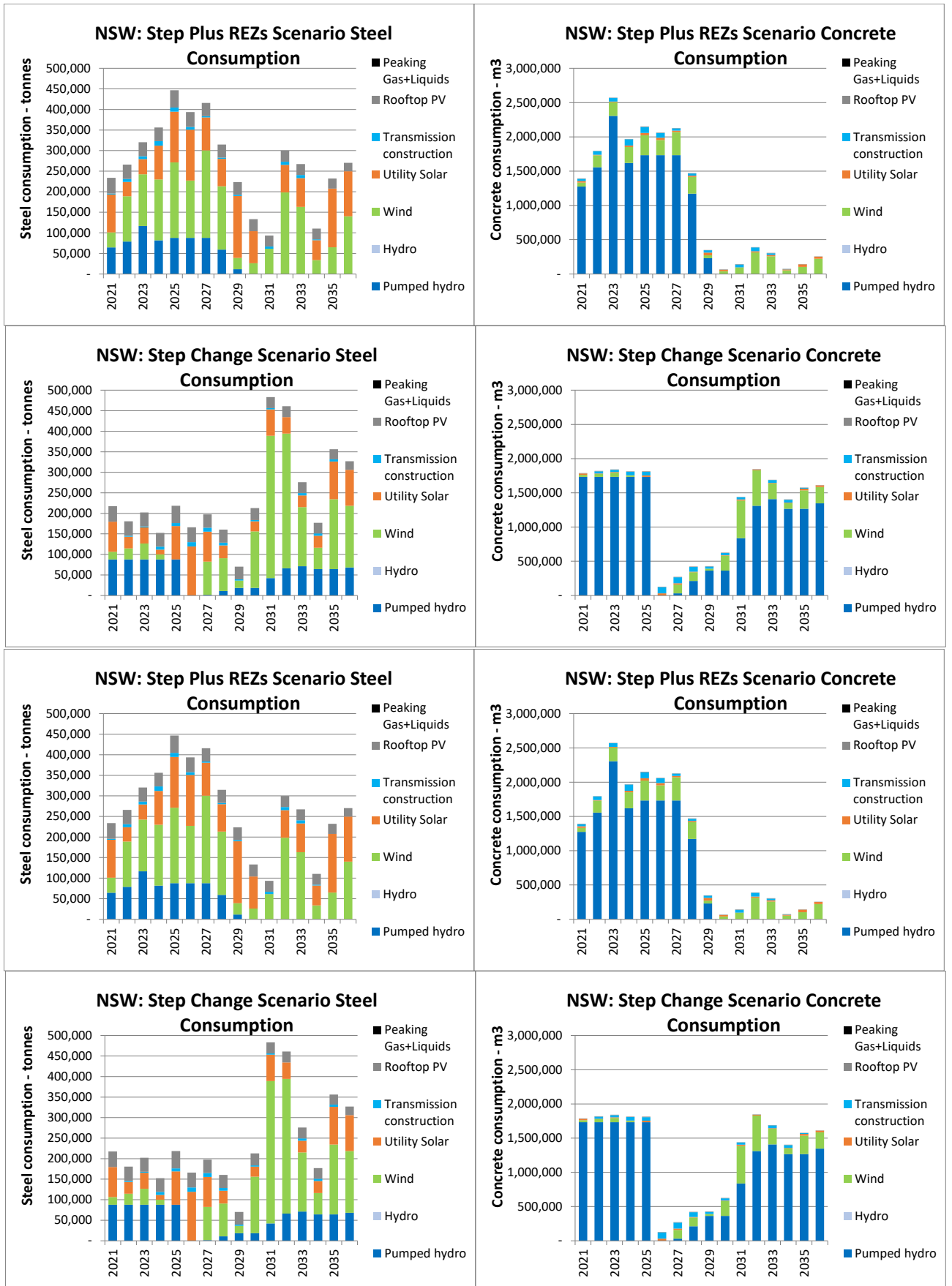
Figure 26: Steel and Concrete Requirements for the Step Change and Step Plus REZs scenarios, 2021-2036
