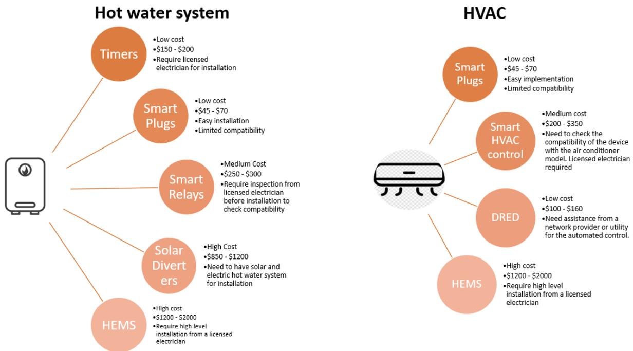
Figure 10 Summary of load flexibility enabling technologies for HVAC and hot water
