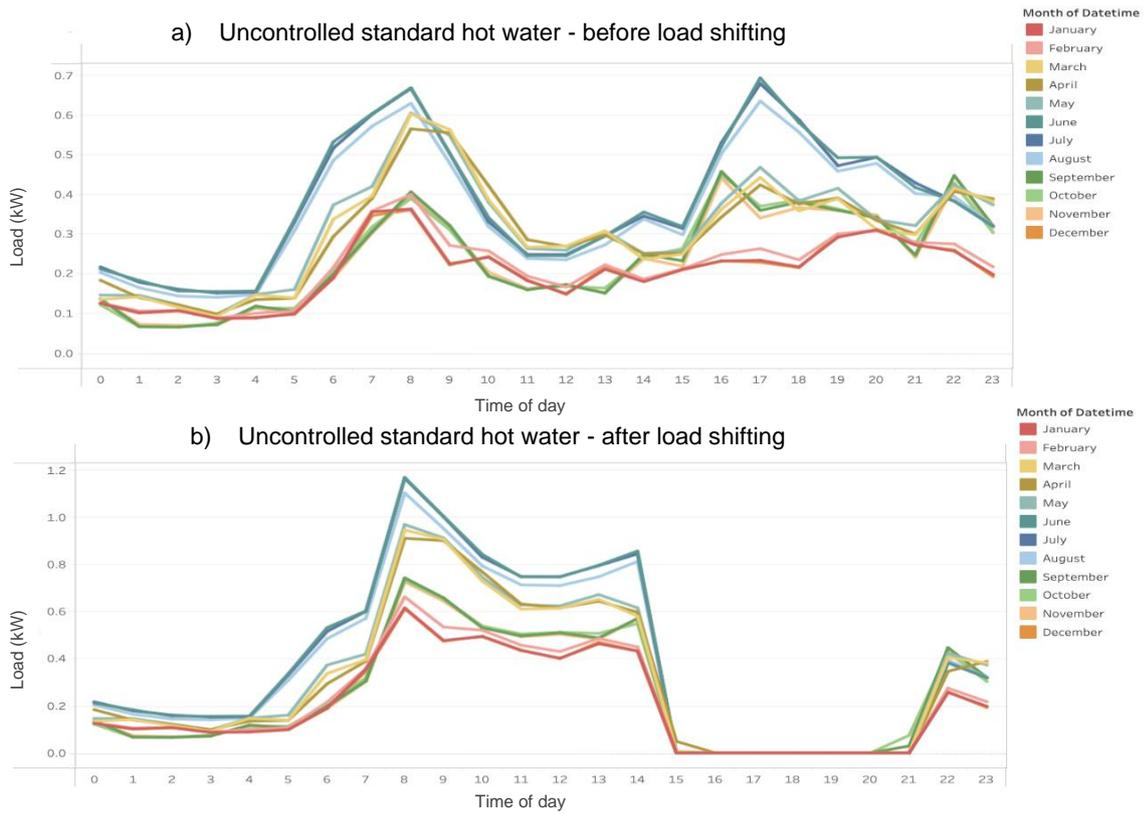
Figure 26 Impact of applying load flex on uncontrolled standard hot water load profile: (note different scales for graphs)
