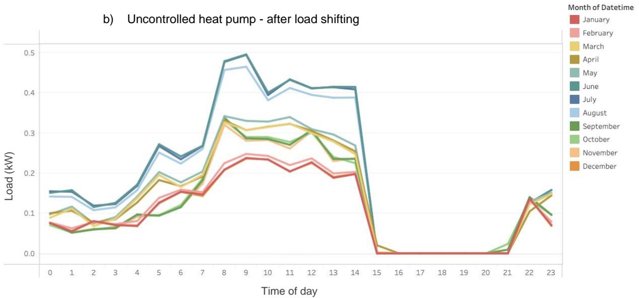
Figure 25 Impact of load flex on uncontrolled heat pump hot water load profile:
