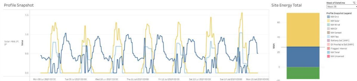
Figure 38 System dynamics for underlying load & controlled solar boost hot water, (a) summer & (b) winter week
