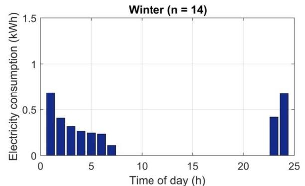
Figure 5 Average hourly electricity consumption per season, controlled standard electric element HW (consumption on a per-occupant basis)
