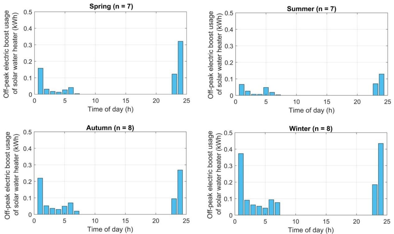
Figure 3 Average hourly electricity consumption per season, electric boost of SWH (controlled) (on a per-occupant basis)
