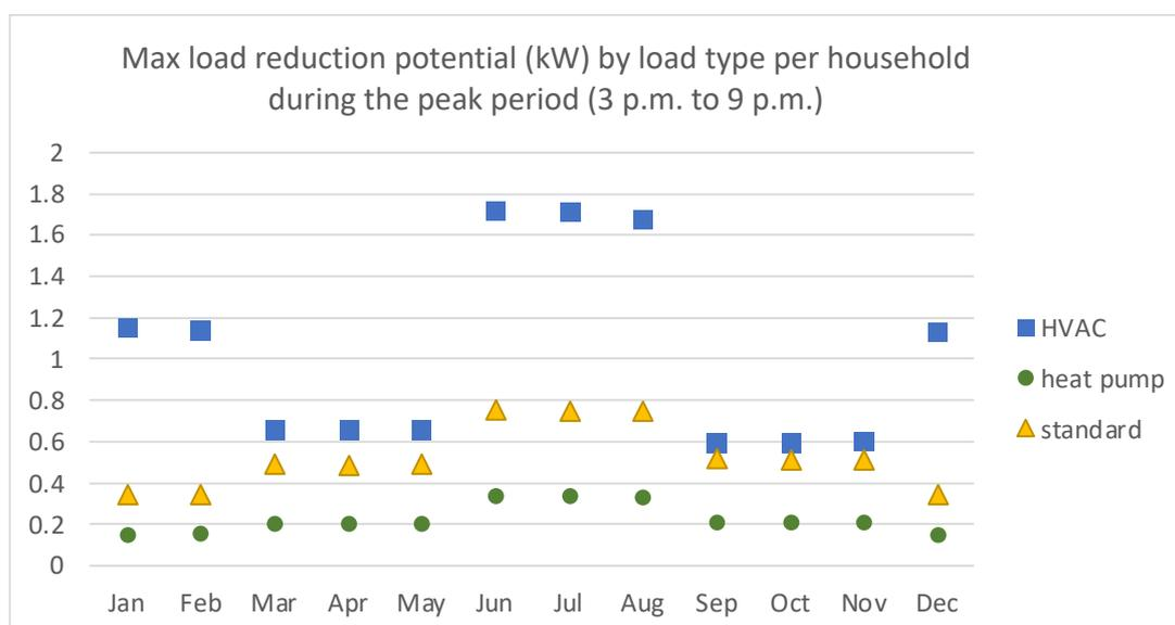
Figure 21 Potential maximum capacity of various flexible load resources at a typical household
