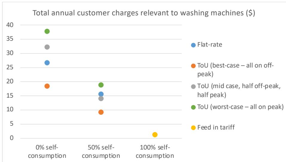
Figure 20 The potential for flexing washing machines to match onsite generation to reduce electricity bills
