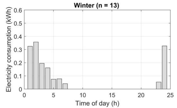
Figure 7 Average hourly electricity consumption per season for heat pump HW (controlled, night) (consumption on a per-occupant basis)
