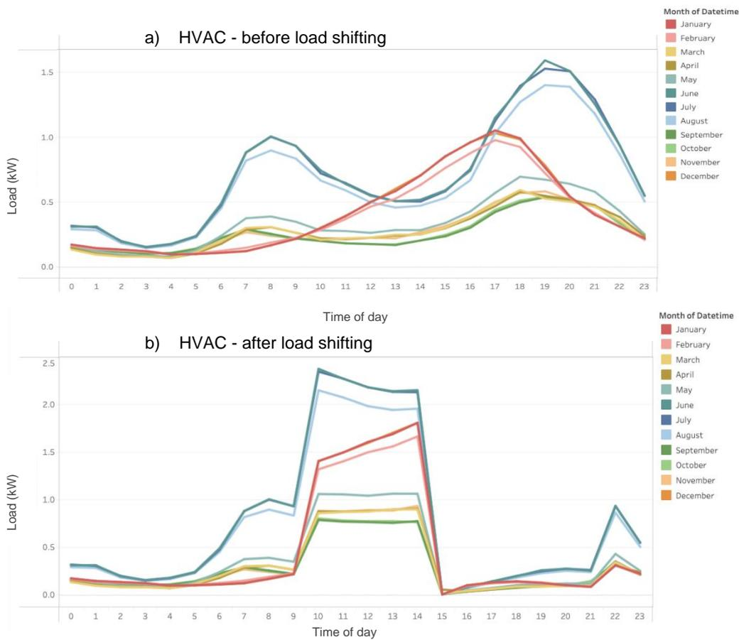
Figure 27 Impact of applying load flex on HVAC load profile: (note different scales for graphs)
