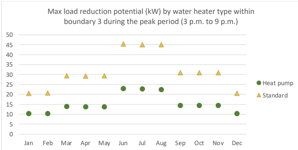
Figure 23 Maximum load reduction potential of various hot water systems in Boundary 3
