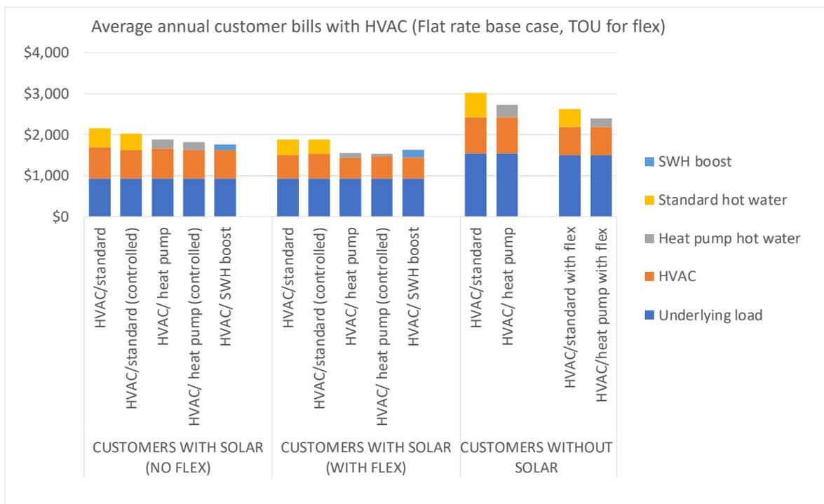
Figure E1 Overview of the impact of load flexibility on customer bills
