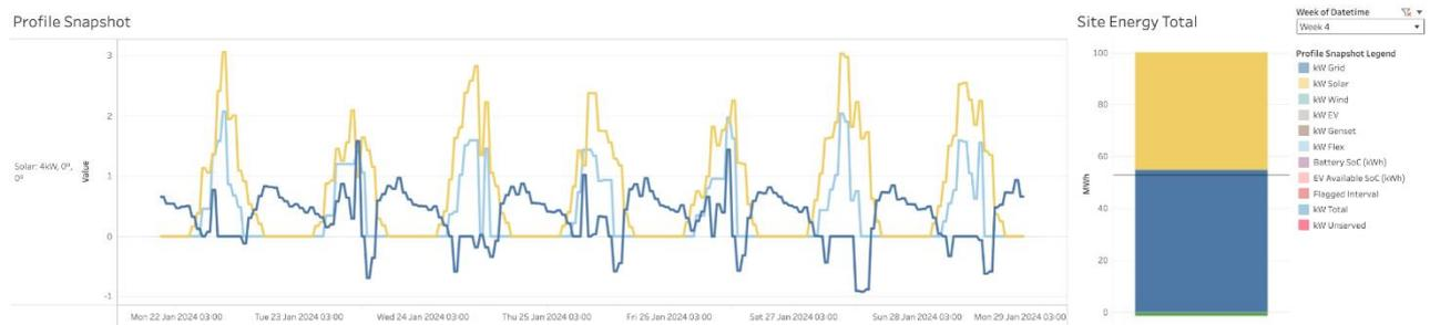
Figure 40 System dynamics for underlying load, HVAC, & controlled heat pump hot water (summer week)
