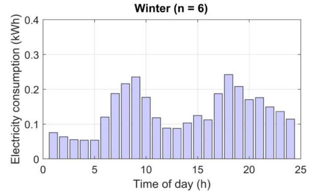
Figure 4 Average hourly electricity consumption per season, standard electric element HW (consumption on a per-occupant basis)
