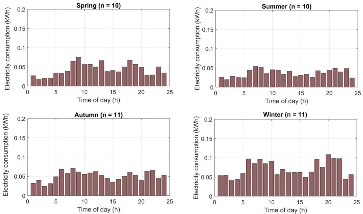
Figure 6 Average hourly electricity consumption per season, heat pump HW (consumption on a per-occupant basis)
