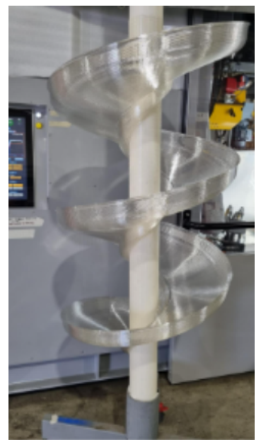
Sidewinder's bespoke 3D printing setup enables dual-material printing, real-time geometric correction and toolpath simulation, without the need for support structures.
