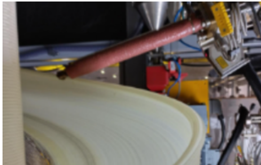
Sidewinder's bespoke 3D printing setup enables dual-material printing, real-time geometric correction and toolpath simulation, without the need for support structures.
